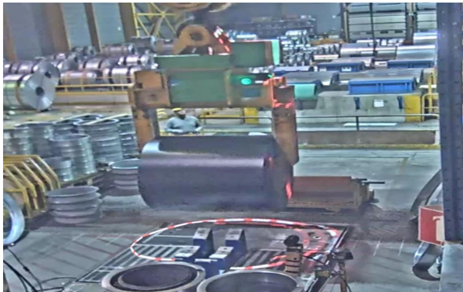
Figure 11. A red-white light projection of a circle beneath the suspended load
