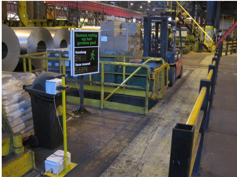
Figure 4. A digital sign displaying the amount of passers-by on the safe pathway
