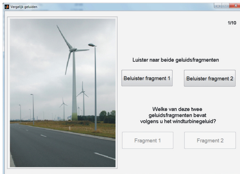
Fig. 6. Computer interface (in Dutch) used for pair-wise comparison of two samples, where one of these contained wind turbine noise.
