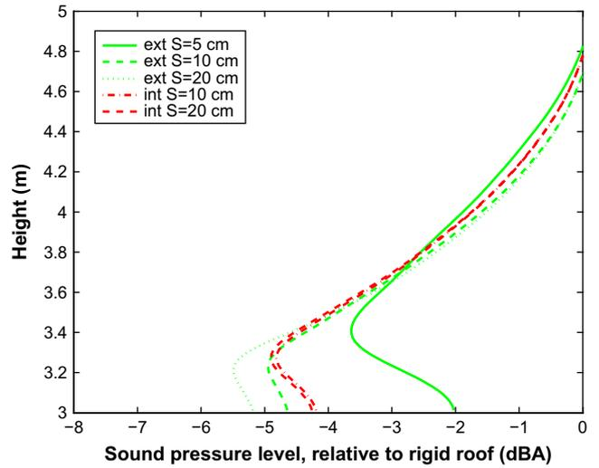
Fig. 5. Sound pressure level, relative to a rigid roof, over the full height of the window at façade B ( $y = 3$  m to  $y = 5$  m). A light vehicle is considered at 70 km/h, in case of the 5-m building extension. Extensive green roofs with substrate thicknesses  $S$  of 5 cm, 10 cm and 20 cm, and intensive green roofs of 10 cm and 20 cm are shown.
