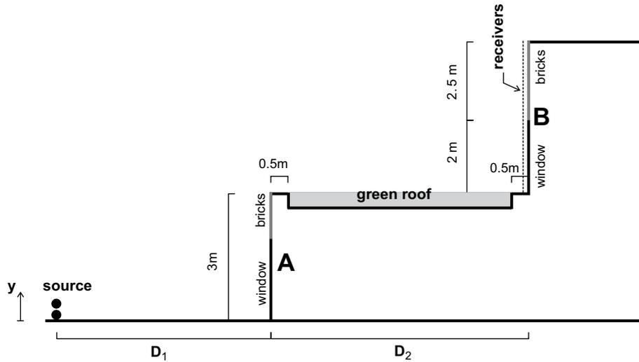
Fig. 1. Representation of a green roof on a building extension (configuration 1). The couple  $(D_1, D_2)$  takes the following values in the numerical simulations: (5,10) and (10,5). Receivers are located along façade B. The window under study is located between  $y = 3$  m and  $y = 5$  m.
