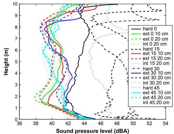
**Fig. 9.** Sound pressure level over the full height of façade C, for a light vehicle at 70 km/h, in configuration 2. Roofs with slopes  $\alpha$  of  $0^\circ$  (flat),  $15^\circ$ ,  $30^\circ$  and  $45^\circ$  are shown, made of rigid materials or with a green roof cover. Extensive green roofs (“ext”) with a substrate thickness  $S$  of 10 cm and 20 cm are shown, and intensive (“int”) green roofs with a substrate thickness  $S$  of 20 cm.
