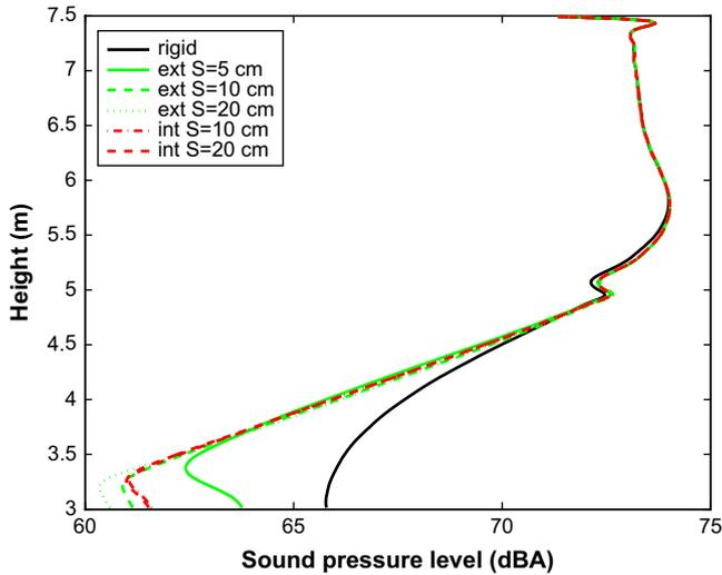
Fig. 3. Sound pressure level over the full height of façade B in configuration 1, for a light vehicle at 70 km/h, in case of the 5-m building extension  $(D_1, D_2) = (10, 5)$ . A rigid roof, extensive green roofs (“ext”) with substrate thicknesses  $S$  equal to 5 cm, 10 cm and 20 cm, and intensive (“int”) green roofs with thicknesses of 10 cm and 20 cm are shown.
