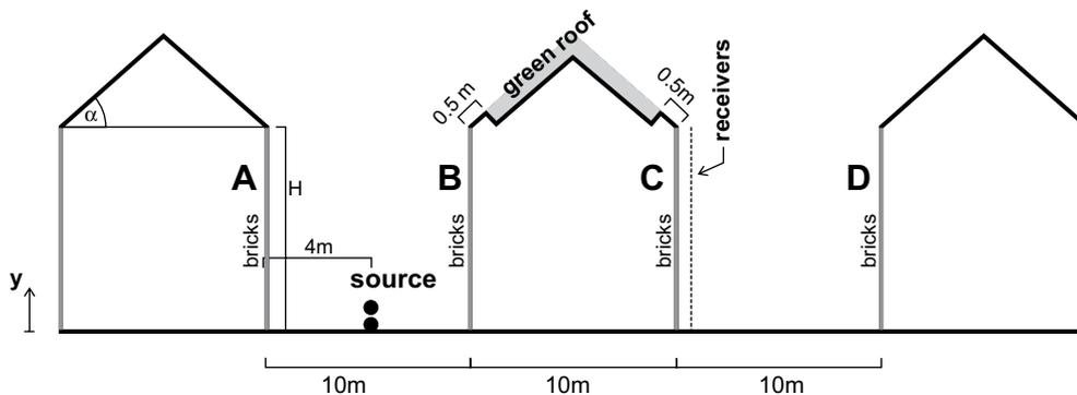
Fig. 2. The idealized street canyon configuration 2. The façade height  $H$  depends on the slope angle of the roof  $\alpha$  (values of  $\alpha$  equal to  $0^\circ$ ,  $15^\circ$ ,  $30^\circ$ , and  $45^\circ$  correspond to values of  $H$  equal to 10 m, 9.33 m, 8.56 m, and 7.5 m). Receivers are located along façade C.
