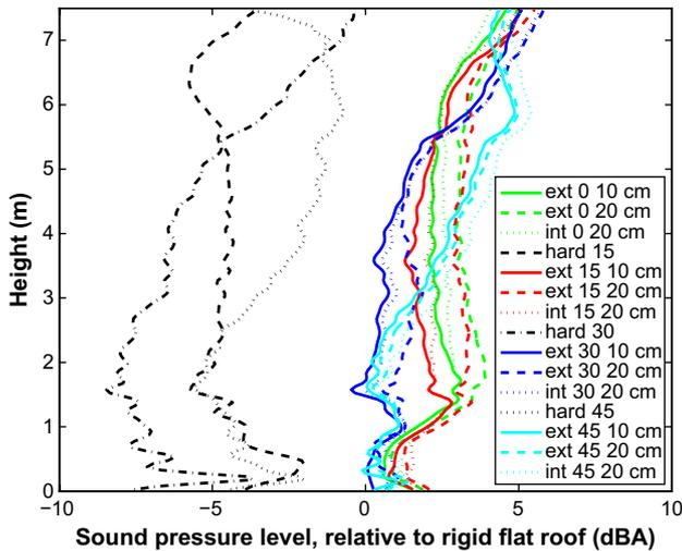
**Fig. 10.** Sound pressure level, relative to a rigid flat roof, over the full height of façade C, for a light vehicle at 70 km/h, in configuration 2. Roofs with slopes  $\alpha$  of 0° (flat), 15°, 30° and 45° are shown, made of rigid materials or with a green roof cover. Extensive green roofs (“ext”) with a thickness of 10 cm and 20 cm are shown, and intensive (“int”) green roofs with a thickness of 20 cm.
