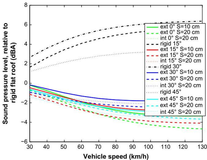
**Fig. 11.** Average sound pressure level, relative to a rigid flat roof, over façade C (from  $y = 0$  m to  $y = 7.5$  m), for a light vehicle in function of vehicle speed (configuration 2). Roofs with slopes  $\alpha$  of 0° (flat), 15°, 30° and 45° are shown, made of rigid materials or with a green roof cover. Extensive green roofs (“ext”) with a substrate thickness  $S$  of 10 cm and 20 cm are shown, and intensive (“int”) green roofs with a substrate thickness  $S$  of 20 cm.
