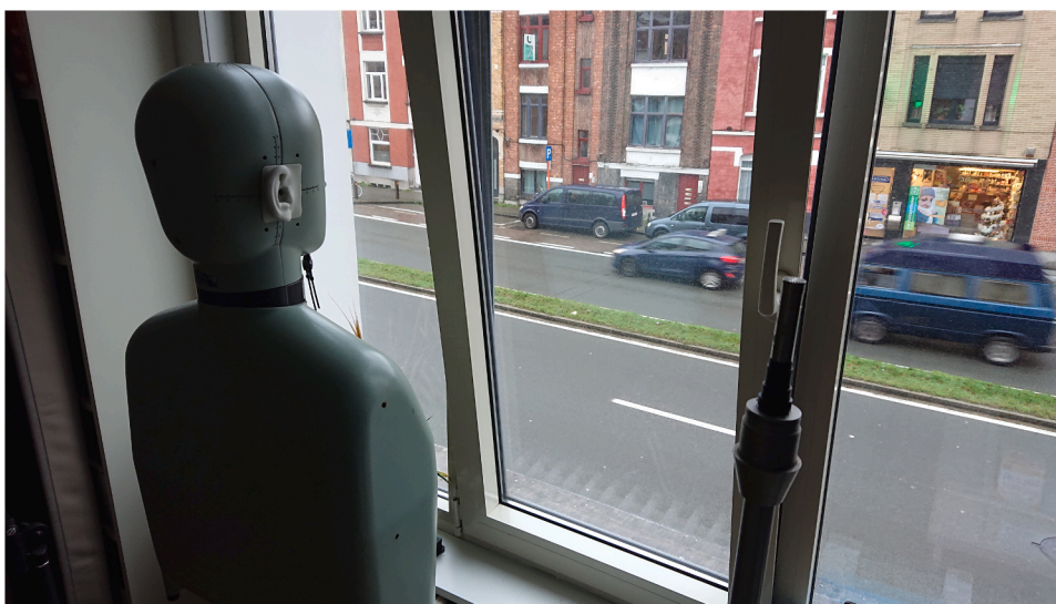
Fig. 2. Photograph of the head-and-torso simulator, measuring binaural road traffic sound, forming the basis for the sound reproduction in the virtual reality experiments. A frontal positioning was chosen in front of a slightly opened window in a real-life setting.
