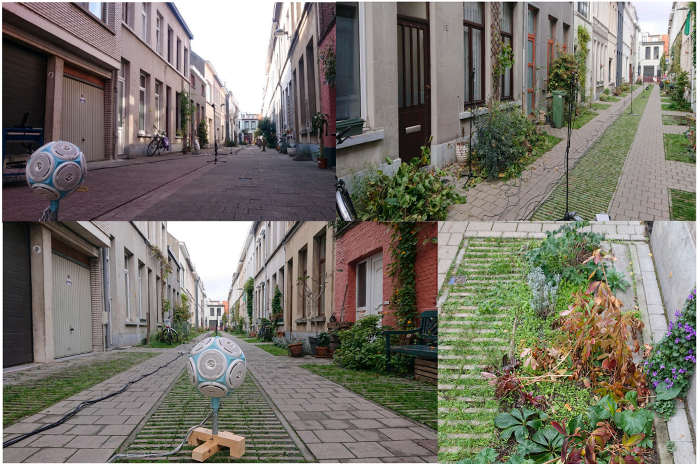
Fig. 2. Photographs showing the street before the greening (upper left), and after the greening interventions (others). The pictures show the dodecahedron loudspeaker used for emitting the test signals (at central positioning, see Fig. 1), the microphones positioned along the length of the street, and a detail of a green patch close to the façade.
