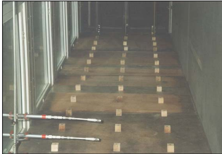
Figure 3.7 Roughness elements, placed before the test section in the wind tunnel, to increase the thickness of the boundary layer.
