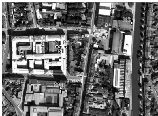
FIG. 2. Ortho photo of the neighborhood of the adjacent city canyons under study. S indicates the location of the loudspeaker, R1 and R2 are the microphones attached to the façades of the building. M0, M1, and M2 are the locations where meteorological parameters were measured above roof level.
