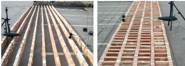
An array of nine parallel walls made from 1440 household bricks loosely stacked on edge (left). The same number of bricks made into a square-cell lattice (right).
