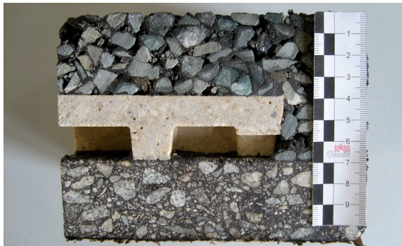
A resonator covered with porous asphalt (left) and the construction of a resonator-improved porous asphalt (right).
