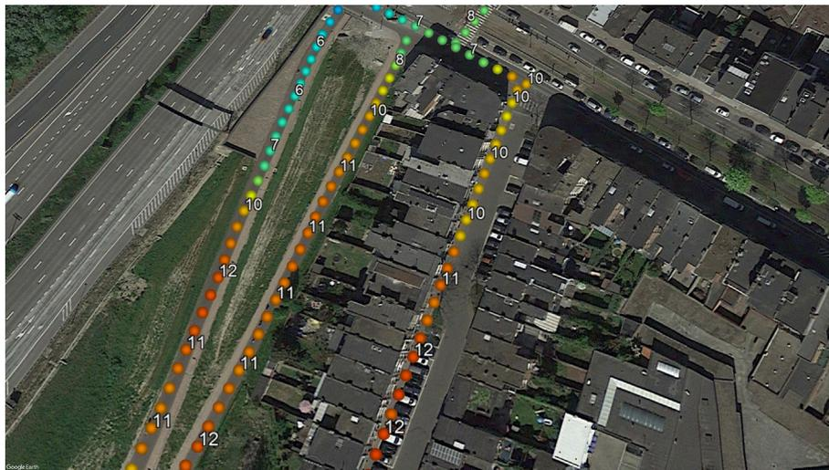
Fig. 11. Detail of  $L_C - L_A$  map (in dB) in the part running towards the underpass below Bridge 2, after the intervention.
