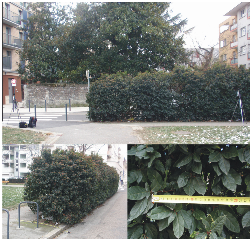
Fig. 3. Photographs showing microphone positioning and hedge details for the controlled pass-by experiment at Grenoble, France (see Fig. 1c).
