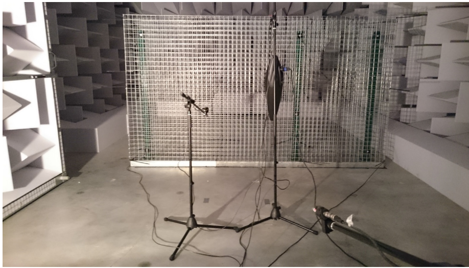
Fig. 3. Photograph of the empty gabion positioned in the semi-anechoic room.
