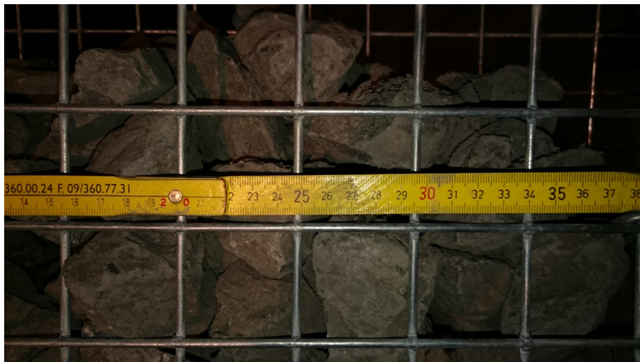
Fig. 1. Photograph of the rigid stones filling up the metal cage.
