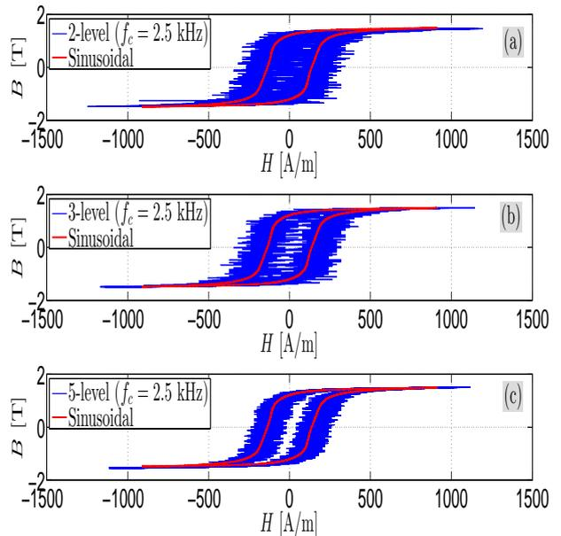
Fig. 5. Hysteresis loops for the 2-level (a), 3-level (b) and 5-level (c) converter topologies, at  $f_c = 2.5$  kHz carrier frequency, compared to the sinusoidal excitation at 1.5 T, 50 Hz. Less minor loops are clear in 5-level converter.
