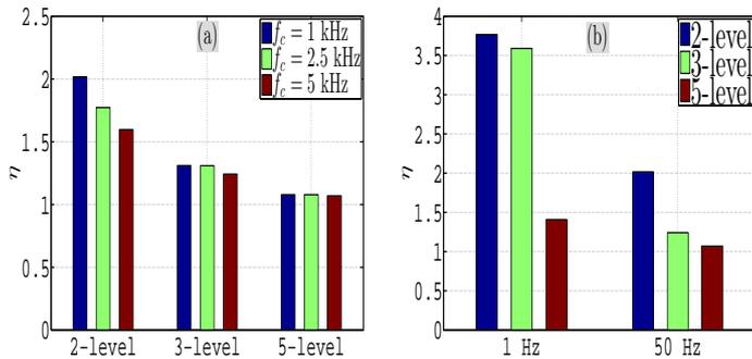
Fig. 7. (a) The increase rate  $\eta$  of the iron loss for the different considered converter topologies at 1.5 T and 50 Hz. (b) The increase rate  $\eta$  of the iron loss, at 1.5 T and 1 kHz carrier frequency, for the different considered converter topologies at 1 Hz and 50 Hz.
