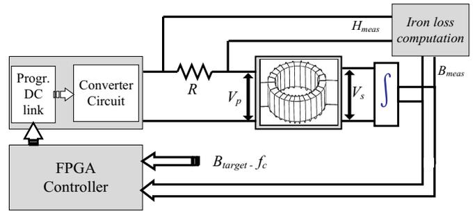
Fig. 1. Overall schematic diagram for a single-line diagram the proposed system.
