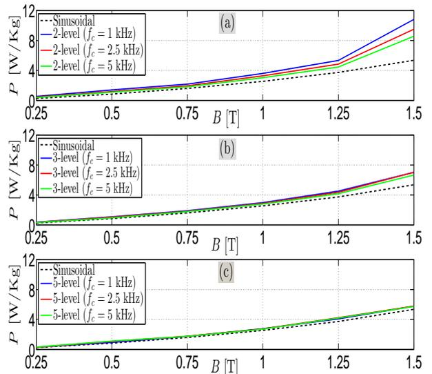
Fig. 6. The measured iron loss for the 2-level (a), 3-level (b) and 5-level (c) converter topologies at different values of the carrier frequency ( $f_c$ ) compared to the sinusoidal excitation at 50 Hz.
