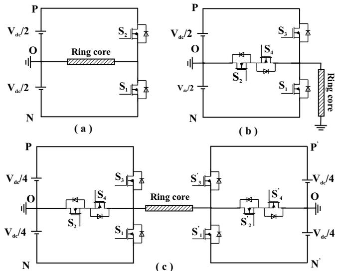
Fig. 2. The single phase circuit of (a) the two-level converter, (b) the T-type three-level converter, and (c) the dual-T-type five-level converter.
