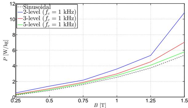
Fig. 4. The measured iron loss for the three considered converters at  $f_c = 1$  kHz compared to the sinusoidal excitation at 50 Hz.
