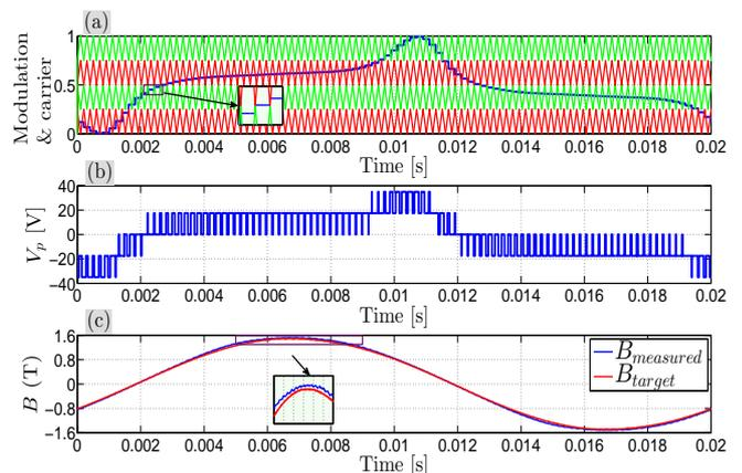
Fig. 3. (a) A comparison between modulation and carrier waveforms, at  $f_c = 5$  kHz, 1.5 T. (b) Single phase of the five-level (dual-T-type) converter output voltage. (c) A comparison between target and measured magnetic induction.
