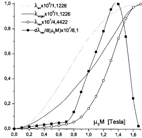
FIG. 1. Measured reversible part of the magnetostriction; anhyseretic and virgin magnetostriction curve obtained from the Preisach model.
