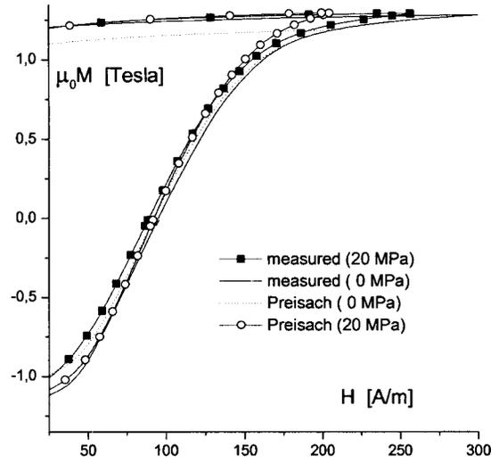
FIG. 4. Comparison of measured and calculated magnetization loop at 20 MPa tensile stress and  $\mu_0 M_{\text{peak}} = 1.3$  T.
