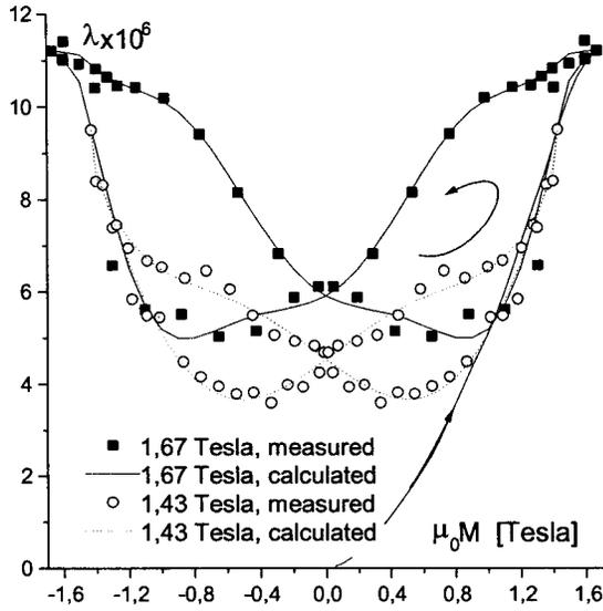
FIG. 3. Comparison of measured and calculated magnetostriction loops.
