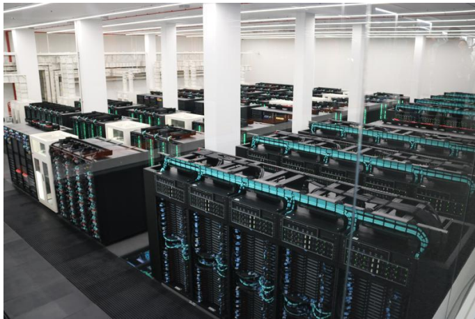
MareNostrum 5 Supercomputer 4480 x NVIDIA H100 GPUs
