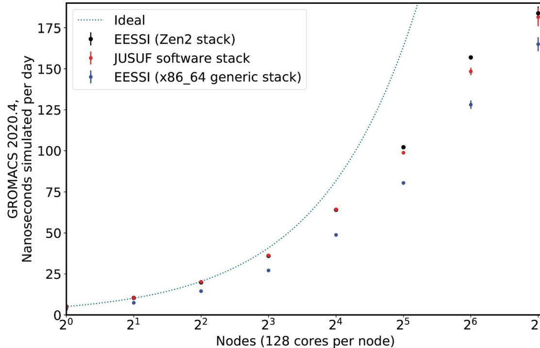
Paper includes **proof-of-concept performance evaluation** compared to system software stack, performed at JUSUF @ JSC using GROMACS 2020.4, up to 16,384 cores (CPU-only)
