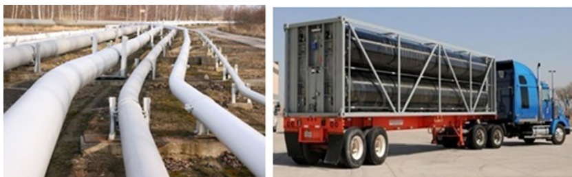
FIG. 2.9 Hydrogen pipelines and hydrogen tube trailers.
