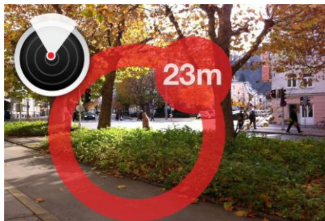
Fig. 2. A screenshot of the AR-based prototype, showing a ring. The distance to the next decision point is shown on the left of the ring to indicate a left turn at the current decision point.
