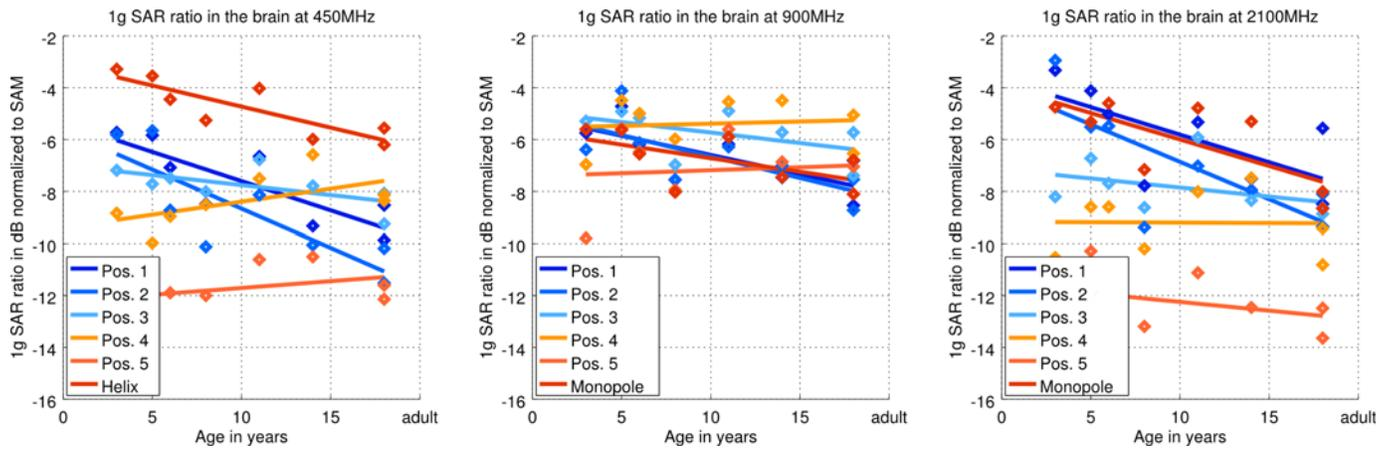
Figure 2. 1g psSAR in the brain tissues of the anatomical models normalized to the 1 g psSAR in the SAM phantom (0dB) for 450 MHz (left), 900 MHz (center) and 2100 MHz (right) and the different generic phones. The markers show the individual results of the anatomical models, and the lines are linear least square fits of these.
