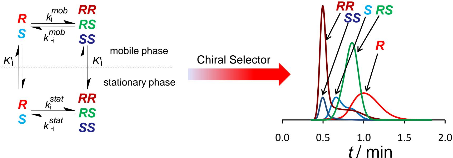
Prediction of unusual elution profiles of enantiomers in non-racemic mixtures on an achiral stationary phase doped with small amounts of a chiral selector
