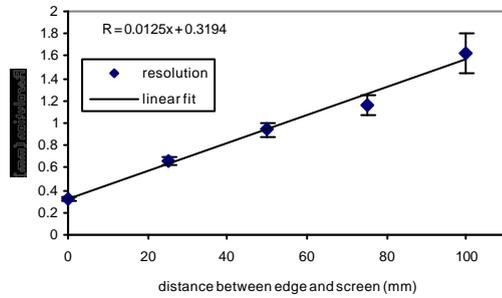
**FIGURE 4.** Neutron radiograph resolution as function of the distance from the conversion screen.
