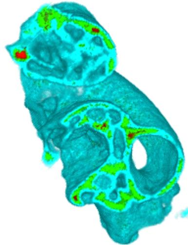
**FIGURE 5.** Neutron micro-tomography of a coral
