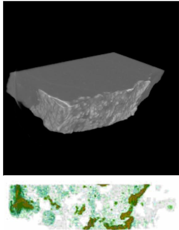
**FIGURE 3.** Reconstruction of the mercury distribution in cinnabar stone from Toscana.
