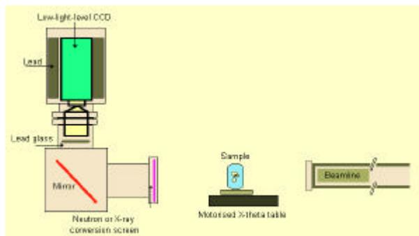
**FIGURE 1.** A schematic representation of the tomography set-up. In the case of neutrons a lens can be placed between the sample and the beam-line. The tomography set-up is completely automated which allows the operator to leave the instrument. When the storage ring needs to be refilled or if there is an accelerator problem the tomography is automatically paused and restarted when the particle beam is back on-line.
