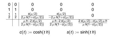
$$lte_{EFLob} = -\frac{h^5}{2880} \left( y^{(5)}(x_k) - \mu^2 y^{(3)}(x_k) - 5 f_y \left( y^{(4)}(x_k) - \mu^2 y^{(2)}(x_k) \right) \right) + \mathcal{O}(h^6)$$
