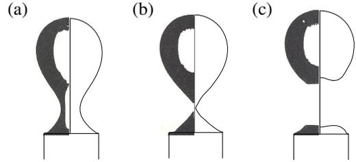
Fig. 2. Comparison of the experimental (left) and numerical (right) bubble shape at (a) -2 ms, (b) at detachment and (c) 2 ms afterwards, for a case studied experimentally by Longuet et al. [5].
