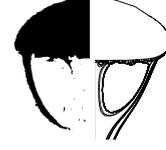
Fig. 1. Comparison of the experimental (left) and numerical (right) steady-state shape of bubble A in Table I from Hnat et al. [3].
