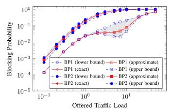
Fig. 4: Blocking probability for a system with S=45 slices and  $n_2=5$ . Random Assignment policy.
