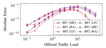
Fig. 6: Absolute error of the blocking probabilities BP1 and BP2 calculated using the approximate Markov chain for the various assignment policies.
