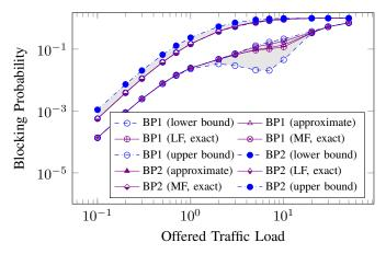
Fig. 5: Blocking probabilities for a system with S=45 slices and  $n_2=5$ . Least Filled (LF) and Most Filled (MF) policies.
