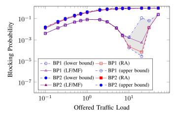
Fig. 8: Blocking probability for a system with S=120 slices and  $n_2=20$
