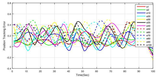
Fig. 3. Motion of following vehicles under our nonlinear unidirectional control law (8). The amplitude of the signal (visually) *stays bounded* when the index of the vehicle increases.
