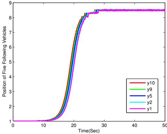
Fig. 1. Motion of ten following vehicles under control law (8) when the leading vehicles follow an integrated soliton solution, which takes the form  $atanh(\cdot)$ . The soliton appears to move backward as the nonlinear reaction of followers transforms ever tinier soliton-compatible fluctuations of their leaders into solitons that switch ever earlier.
