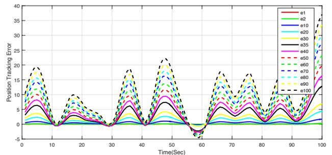
Fig. 4. Motion of following vehicles under the linear unidirectional control law (12). The amplitude of the signal (visually) *increases* when the index of the vehicle increases. It has been proven [5], [7] that this behavior is unavoidable for any linear controller.
