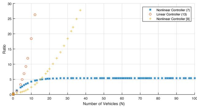
Fig. 5. First-to-last ratio  $R_{FTL}$ . Comparison of nonlinear and linear controllers of a network of 100 agents with random inputs of typical amplitude  $\delta_0 = 0.5$ .
