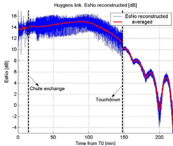
Fig. 3. Huygens in-flight data from the Automatic Gain Control AGC, converted into power to noise ratio,  $E_s/N_0$ .
