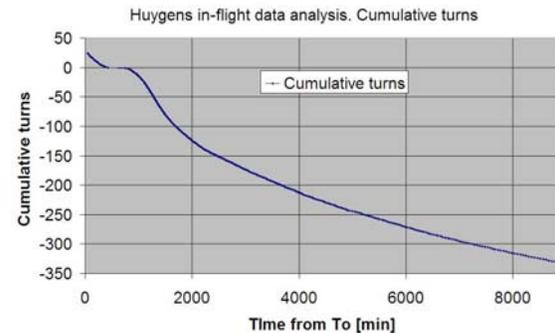
Fig. 7. Reconstructed cumulative turns during the Huygens descent, from link establishment until touchdown. The Huygens Probe completed 24 rotations in the CCW direction and 330 rotations in the CW direction.
