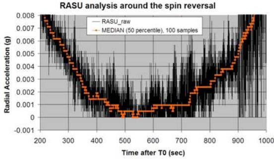
Fig. 10. The RASU median method. RASU data is cut at 0g. The raw data reflects noisy attitude disturbances around the centrifugal mean force (due to spin). The median value (non smoothed) is a good estimator of the centrifugal force.
