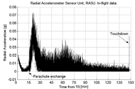
Fig. 2. Huygens in-flight raw data from the Radial Accelerometer Sensor RASU. Note the data is trimmed to zero. The touchdown shock is captured.
