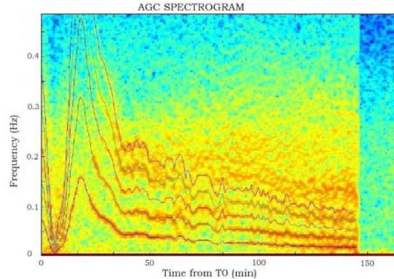
Fig. 9. The spectrogram of the AGC signal. The AGC-FFT method is used to derive a filtered spin rate (superposed lines) from the raw AGC signal. Some of its harmonics also appear in the FFT.
