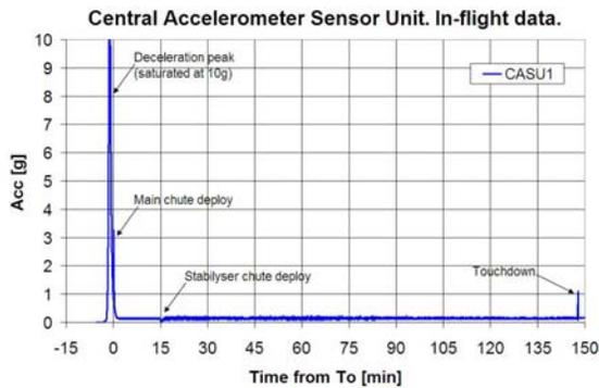
Fig. 1. Huygens in-flight data from the Central Accelerometer Sensor CASU 1. The main events of the mission are captured in the graph: main deceleration peak, main and stabilizer chutes deployment, and touchdown.
