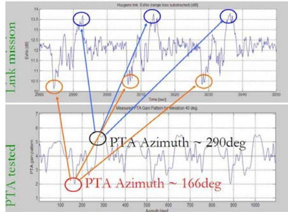
Fig. 6. The AGC manual counting method, used to derive the absolute azimuth (in Probe body fixed axis) by comparison of the AGC signal (upper graph) and the antenna measured patterns (bottom graph).
