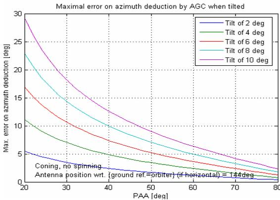
Fig. 8. Error estimates in Huygens azimuth (in Titan's local frame), implied by the assumption of a Probe vertical, for several actual inclinations of the Probe horizontal plane.
