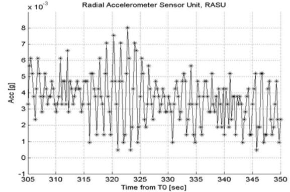
Fig. 4. RASU zoom-in. An oscillation of  $\sim 0.8$  Hz is observed on top of the nominal centrifugal force (due to spin).
