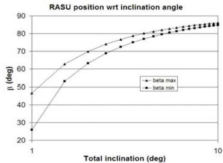
Fig. 13. Constrains in the Huygens  $\beta$  angle (angle between the RASU radial position in the Probe and the maximum inclination direction) on the surface. X axis is logarithmic. The 2 curves delimits the resolution errors (in the quantization of the raw values and  $g_{\text{titan}}$ ).
