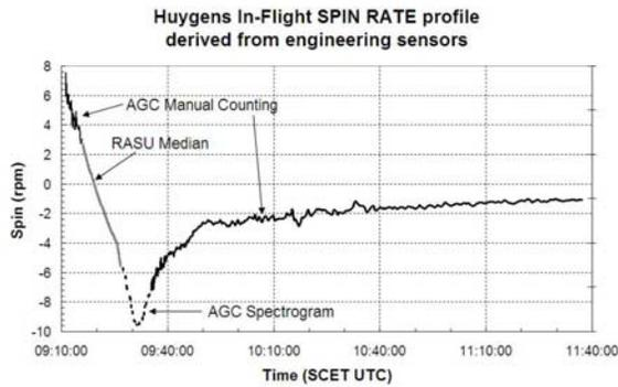
Fig. 11. Reconstructed spin profile: the RASU median method is used around the spin inversion, the AGC spectrogram in the peak, and the AGC manual counting otherwise.
