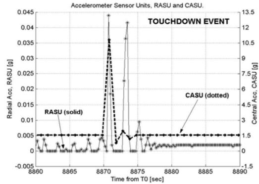
Fig. 12. Touchdown signature in CASU (dotted) and RASU (solid). Please note the different scales. After the peak shock, a 7-8 seconds transient is observed.
