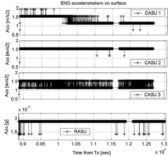
Fig. 16. Surface phase as measured by the Huygens central and radial accelerometers (CASU and RASU).
