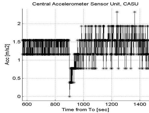
Fig. 5. CASU data at parachute exchange. A calm descent is observed under the main chute (variation of one LSB, due to quantization:  $g_{\text{titan}}$  is nominally  $1.354\text{m/s}^2$ ). A rougher descent occurs with the stabilizer chute (5 LSB change!).
