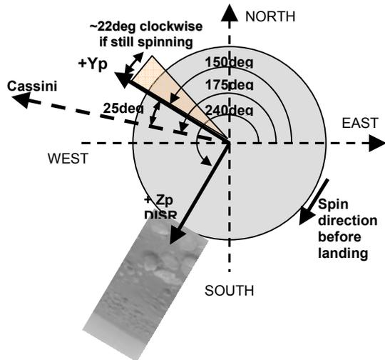
Fig. 15. Estimated landing orientation from the AGC data. According to the analysis, the DISR cameras should be looking in the S-SW direction.
