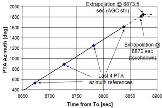
Fig. 14. Azimuth estimation after landing, based on the AGC data. The 4 last AGC-derived azimuths are extrapolated at 8870sec time (official touchdown event) and 8873.5sec (AGC freezes). The 0 azimuth corresponds to an arbitrary integer number of 360 deg.
